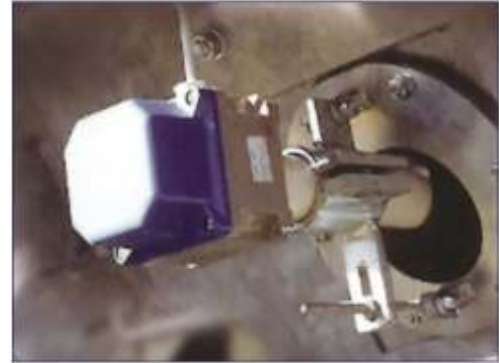
MOISTURE PROBE : Moisture probe for automatic moisture compensation of aggregates - Resistive type or Microwave type.
