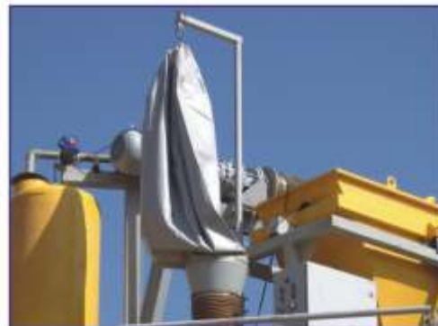
AIR BAG : Airbag eliminates cement dust.
