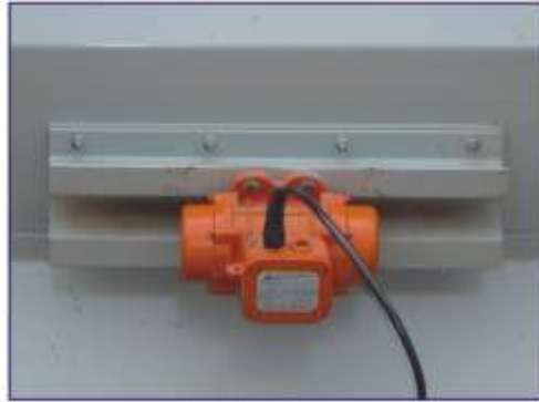
VIBRATOR : Vibrator ensures complete discharge of cohesive material. Vibrator system isolated from main frame.
