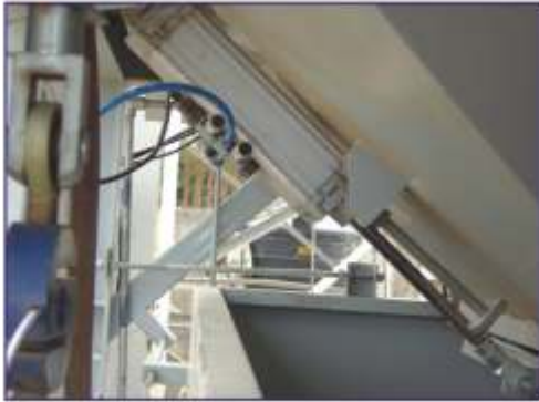
BIN DISCHARGE : Large gates for fast bin discharge. Spilling cycle ensures batching accuracy.
